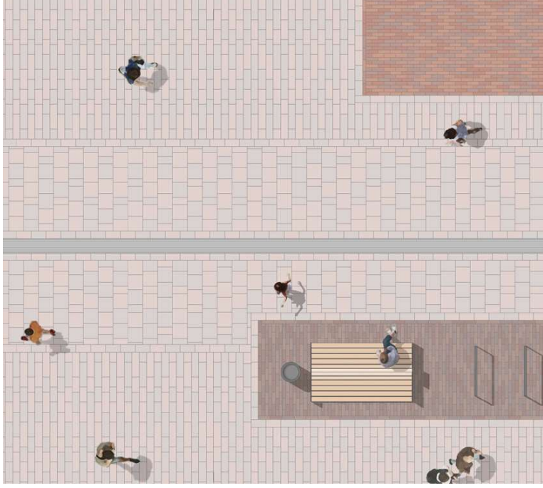
V 2 Betonsteinpflaster Formate: 30/15, 40/15, 50/15, 30/30, 15/30cm
